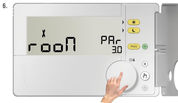
Push the knob or the button "OK" in order to exit the edit mode of the selected parameter. To **continue** the configuration of the other parameters **repeat from point 3.**
