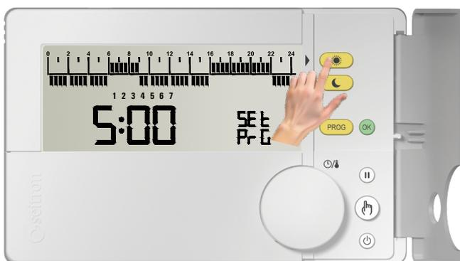
Push "☀️" to set the **comfort mode** (on the time histogram, a segment is shown on the upper strip).
