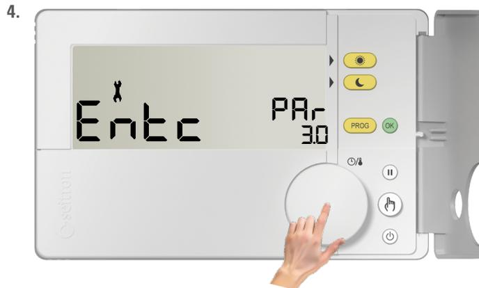
Push the knob or the button "OK" to edit the parameter shown on the display.
